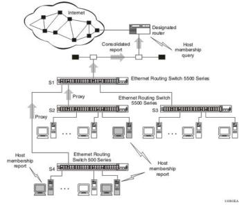
5500 Series switch filtering IP multicast streams (1 of 2)
